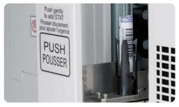
With a dedicated STAT position available the Pentra C200 allows you to add samples at anytime during routine use. The **Pentra C200** combines the power of high capacity automation (192 tests) with the flexibility of STAT access.
